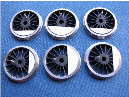
This picture shows the completed wheels with crankpins and balance weights.
