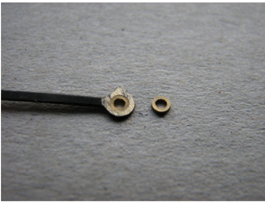
Bush in rod ready for soldering.
